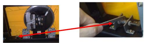
Turn it down to reduce the resistance. Backwards is to increase the resistance.
