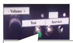
Step 1: Press "Test" button, and go to the setting menu.
