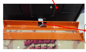
Connect the cable and fix the connecter plate to the cabinet with screws.
