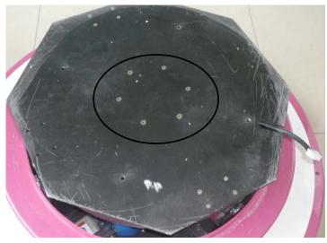
**Step 5** Unplug the connecter and release the tie underneath the black plate.
