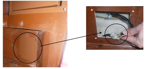
**Step 2** Remove the 4 screws on the rubber pad as indicated in the picture below:
