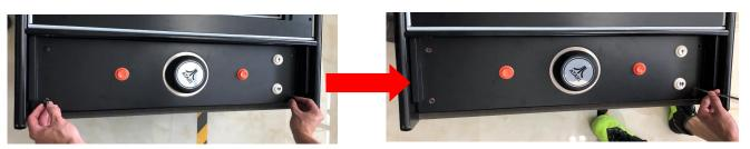
Step 3 Open the control panel as shown. Unplug the connector as indicated by the red circle.
