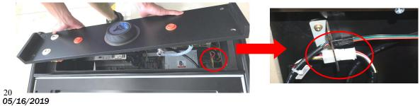
**Step 4** Remove the corner screw covers and loosen the screws.
