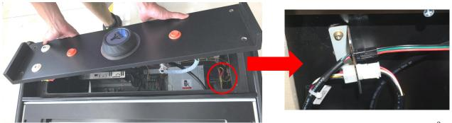
**Step 4** Locate the Power supply. Toggle the switches to 230V.
