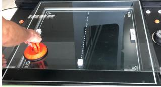
Step 2 Open end panel of player position shown in the pictures. Remove the screw covers and loosen the screws.
