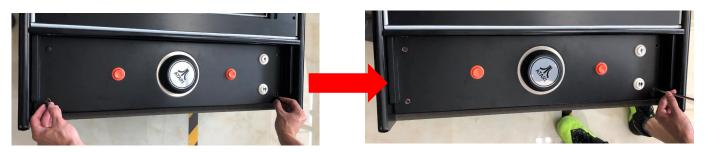
**Step 3** Open the control panel as shown. Unplug the connector as indicated by the red circle.
