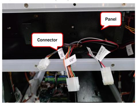
Step 4 Utilize screws to secure Panel.(From cabinet inside)
