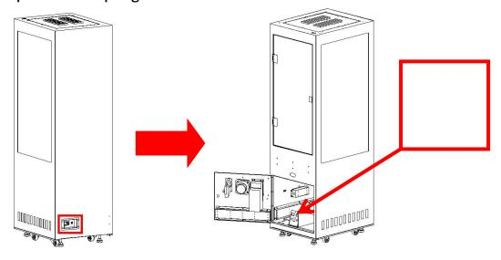
Step 2 Take Control panel out. Locate Control panel assy. Loosen screws to remove Panel plastic.
