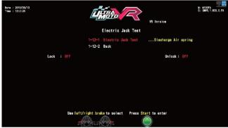
Step 2 Press the [Start] button to start the test. If the Jack mechanism don't move, it means Jack mechanism motor or motor PCB board wrong. Replace motor or motor PCB board.
