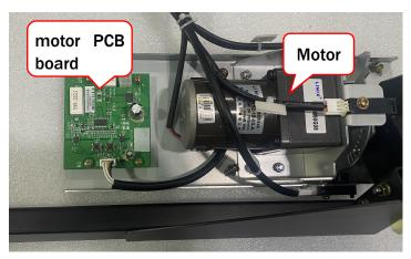
Step 3 If the Jack mechanism moves, but there's still ELECTRIC JACK ERROR. It means the Sensor or the blocking plate wrong.
