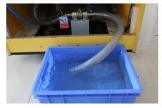
(2) Counterclockwise spin drain SW to drain water.
