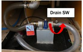
After draining the water, close drain SW, replace hose and assure no leaks.
