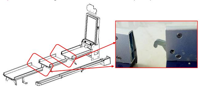
Step 6 Match the red circle area and install the ball slot part on the machine as picture
