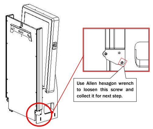
**Step 2** Erect t1he lane bracket, spin the support bar to fix it, then attach the screws as picture shown to fix the lane.
