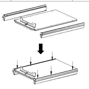
**Step 4** Install the ball slot part by Phillips screwdriver as picture shown.
