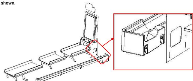
**Step 7** Use Phillips screwdriver Install the marquee part on the machine as picture shown.
