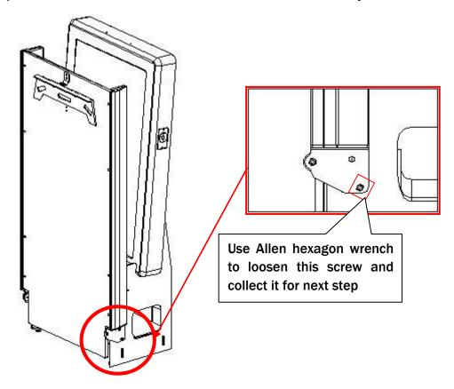
Utilize Phillips screwdriver to loosen the screws to remove the original bracket, and replace the new bracket.
