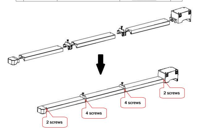
**Step 5** Use the Allen hexagon wrench to lock the extended lane part as picture shown.
