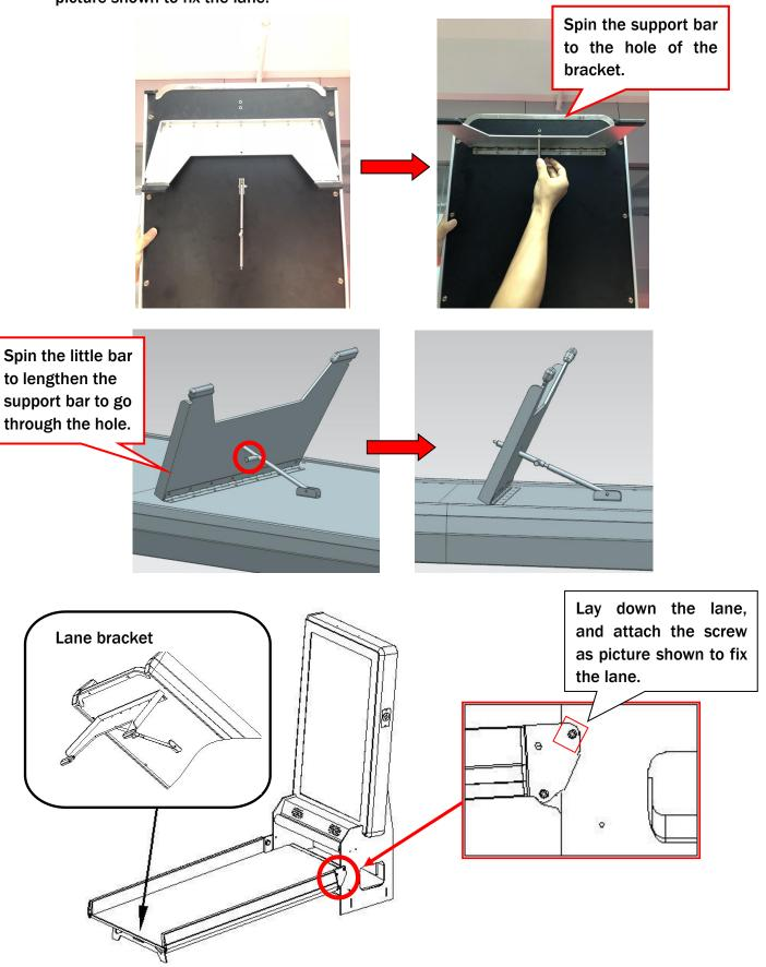
**Step 3** Install the extendeded lane part by wrench as picture shown.
