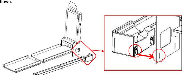
**Step 7** Use Phillips screwdriver to install the marquee part on the machine as picture shown.
