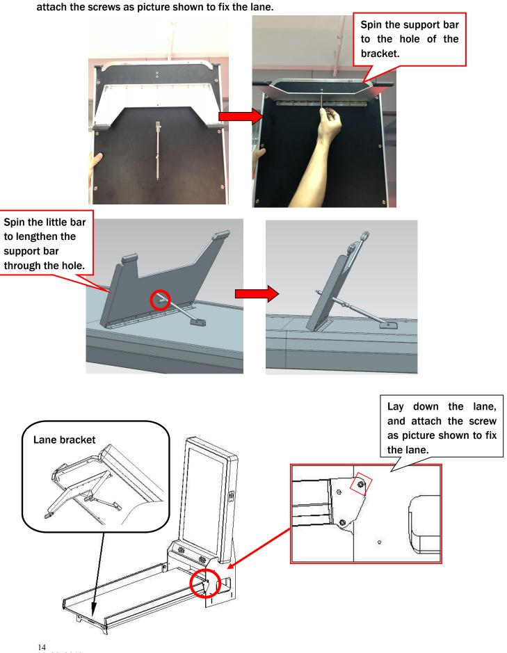
**Step 3** Install the extended lane part by wrench as picture shown.
