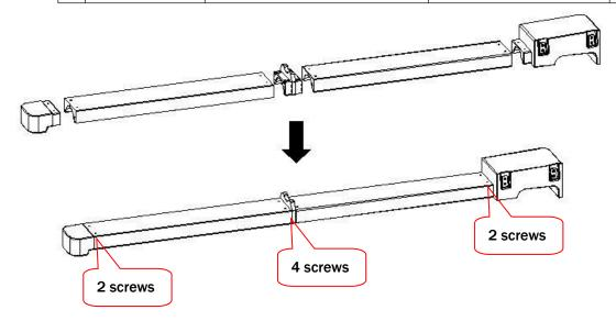
**Step 5** Use the Allen hexagon wrench to lock the extendeded lane part as picture shown.
