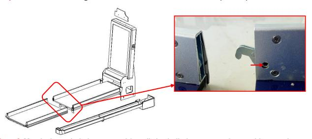
**Step 6** Match the red circle area and install the ball slot part on the machine as picture shown.
